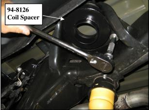
7. Reinstall the rear spring assembly into the rear axle spring perch. Make sure the pigtail of the spring and **OE** isolator properly indexed in the mounting pocket.
