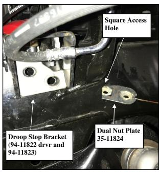
18. Install the droop stop bracket (94-11822 drvr and 94-11823 pass) to the frame and secure using the supplied 12mm X 30mm bolts and washers. Torque the 12mm bolts to 55 ft./lbs.
