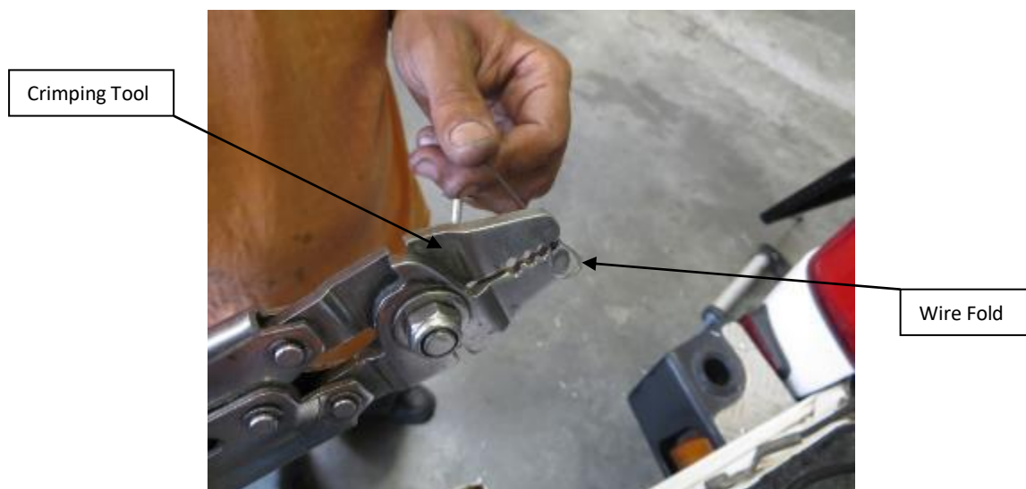
Figure 13: Crimping wires together
