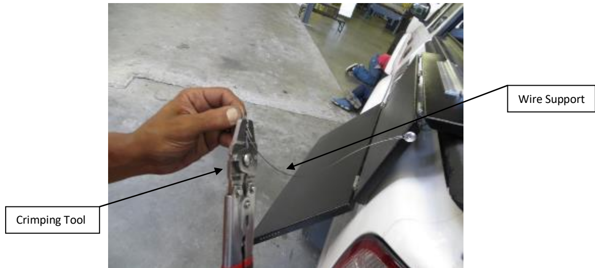
Figure 16: Crimping other end of wire support
